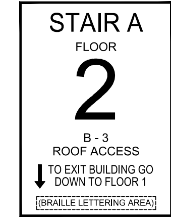
INTERIOR STAIR SIGNAGE EXAMPLE
